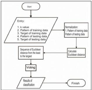
Fig. 3.kNN algorithm flowchart
