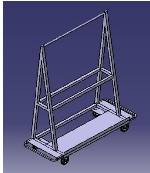
Fig. 5. Design of a Push Aid with Normal Base Size
