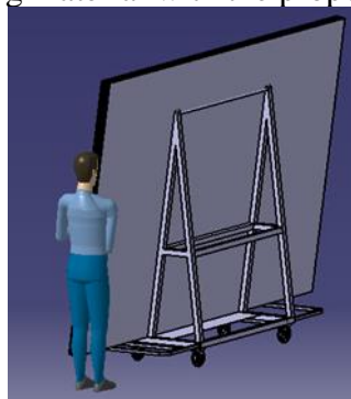
Fig. 7. Process of Transferring Raw Materials with Push Aid Devices
