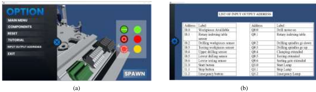
Fig. 4. Added input output address menu (a) List of menu, (b) List of input output address
